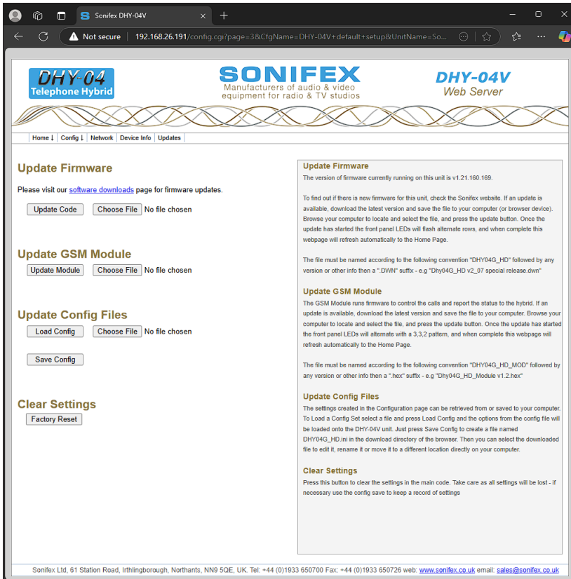
Figure 6-10: Updates Page – to update the system firmware and load/save configuration files
